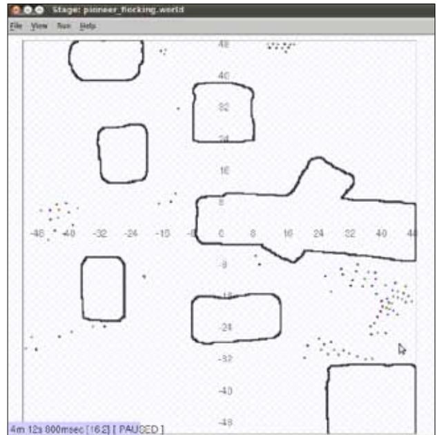
Figure 1: Multi-coloured pioneer robot models forming swarms
